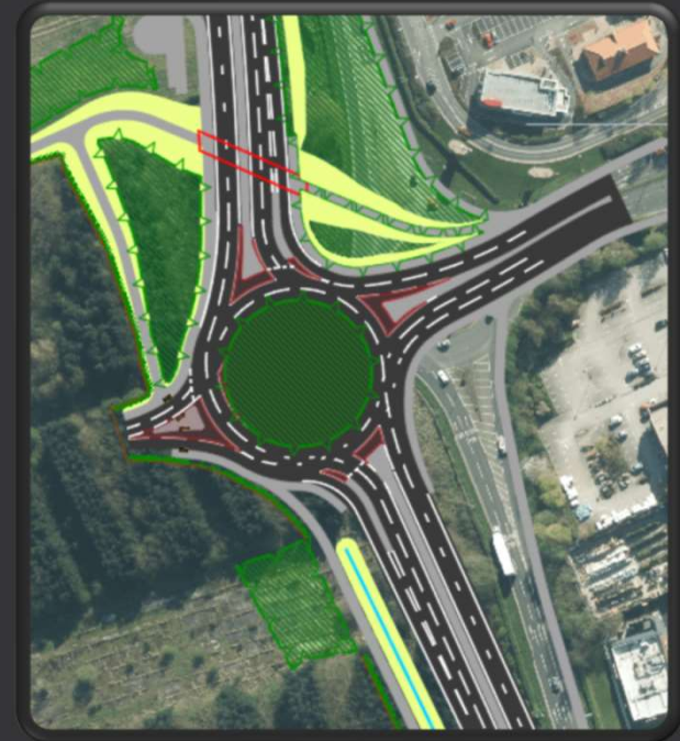
Clifton Moor Roundabout – Proposed Works
